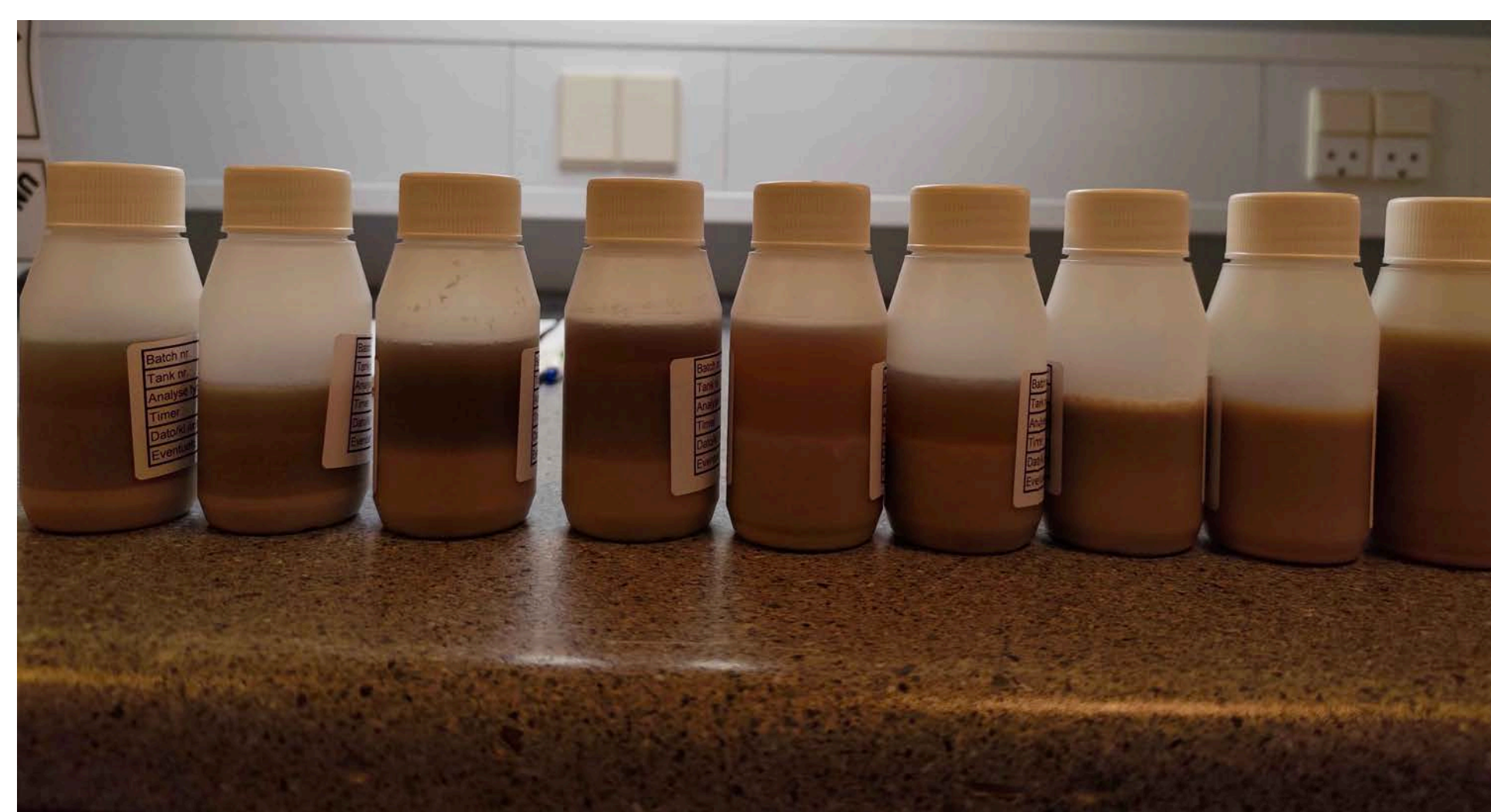
Samples taken from the bioreactor show the change in content of the different fractions during fermentation and the heterogeneity of the environment in the bioreactor.
